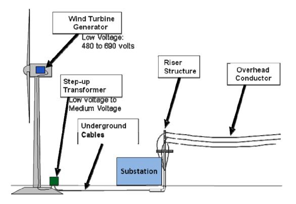
Figure 3-3. Typical Wind Collection System Arrangement.
