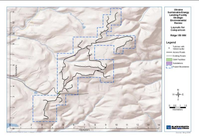
Figure 3-11. Representative Project Configuration (150 MW) on Ridgeline.
