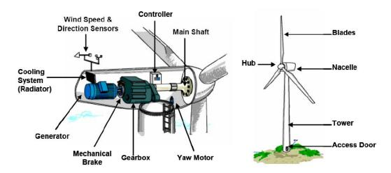
Figure 3-1. Typical Wind Turbine Schematic.
